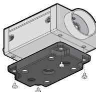
The ASA and ISO-compliant tripod mounting bracket attaches to the camera using the included screws.
