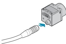
GPIO is used for power, trigger, pulse width modulation, serial input output, and strobe.
