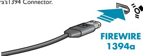
**NOTE:** The camera relies on the 6-pin 1394 cable to provide power. If using an interface card other than that provided, ensure that adequate power is provided.
