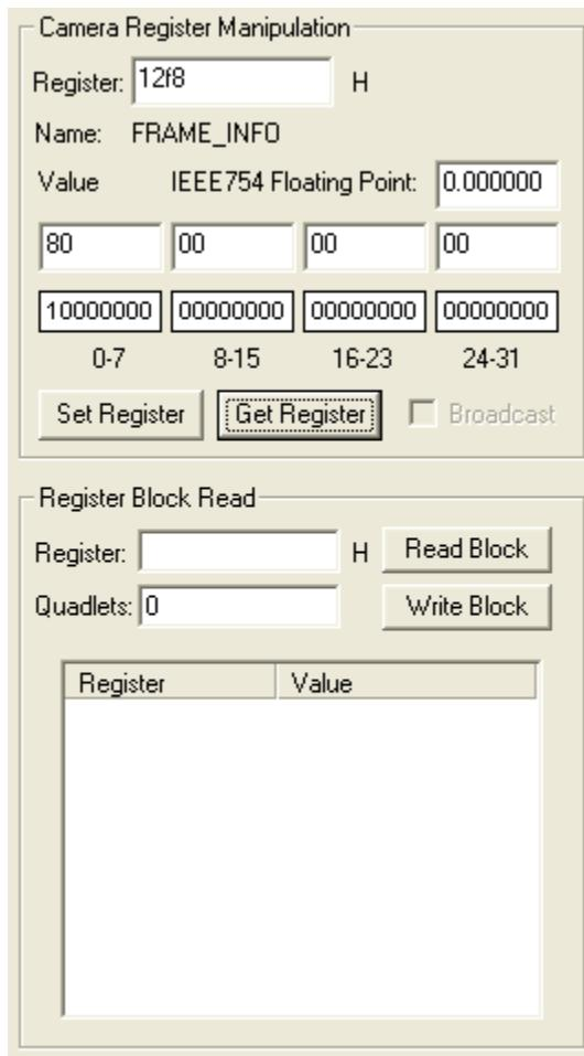
2. Change any or all of bits 22 – 31 to 1, depending on the metadata you want to embed, and which bits are supported by your camera. For more information, consult the *Point Grey Digital Camera Register Reference*. For example, to embed Exposure and Brightness quadlets, set bits 27 and 28 to 1.
