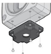
The ASA and ISO-compliant tripod mounting bracket attaches to the camera using the included plastic screws.
